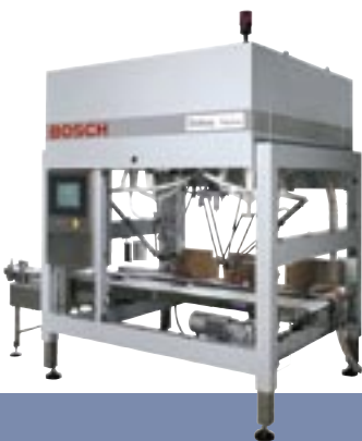
Doboy Robotic Paloma Top Loading Machine places products into cartons.
