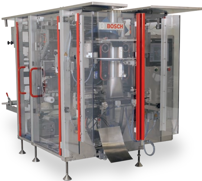
SVE 3600WR Vertical-Form-Fill-Seal Bagger
