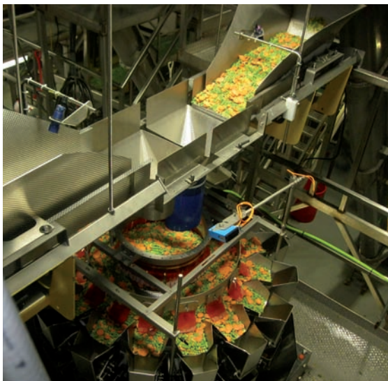
16 Head Yamato Scale weighing mixed vegetables into a Bosch SVE 3600 WR VFFS machine
