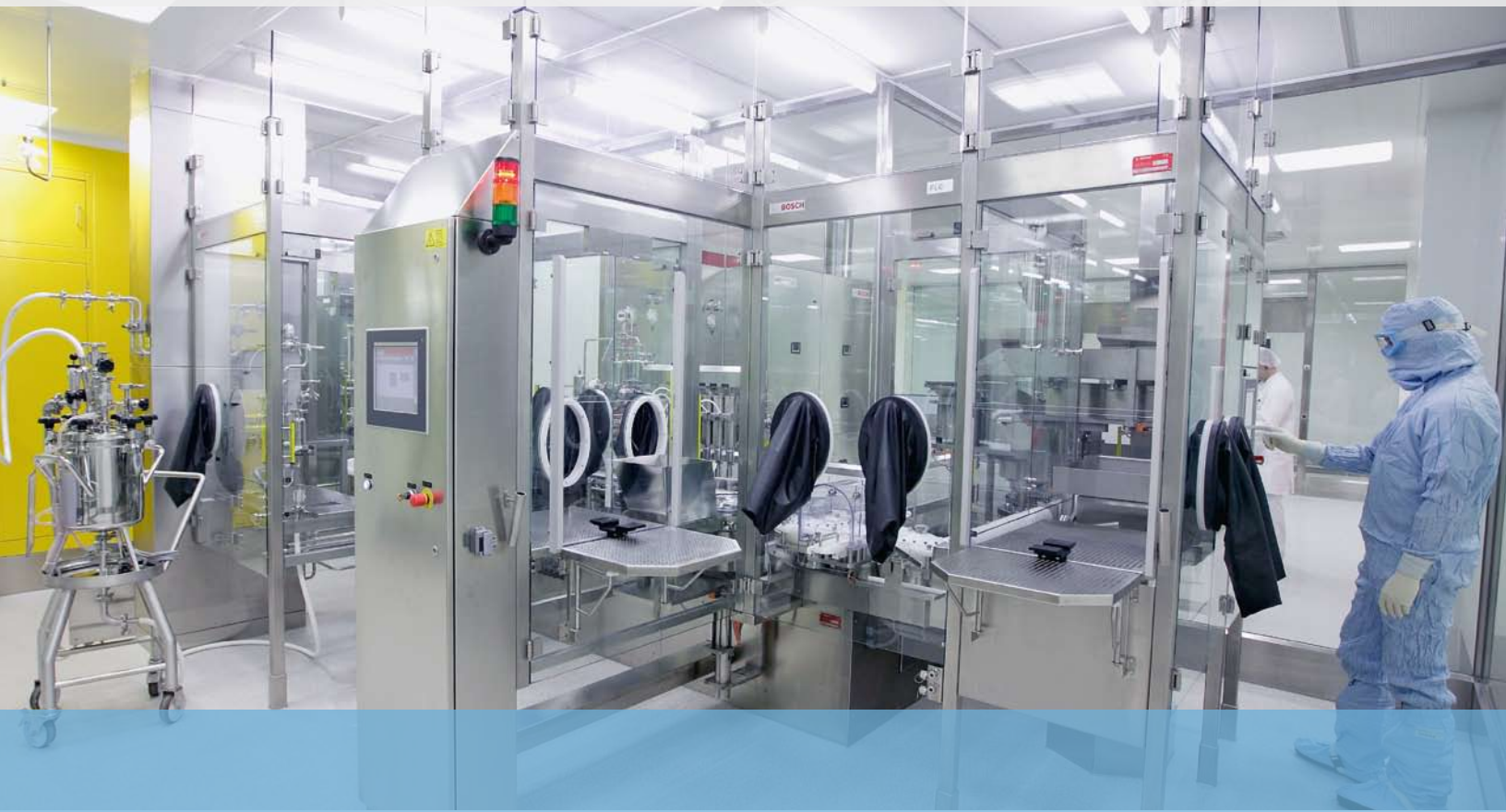
Vial filling and closing machine FLC 3060 with RABS at hameln pharma
