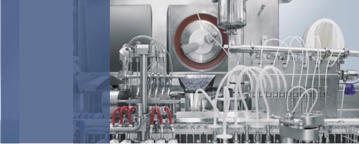
Interior view FLS in isolator
