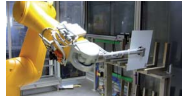
Fig. 5: Handling robot with test panel
