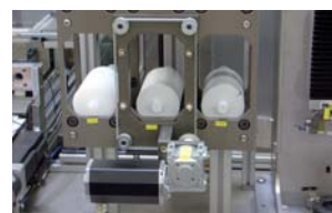
Fig. 4: Storage of sedimenting raw materials (syringes continuously rotated)
